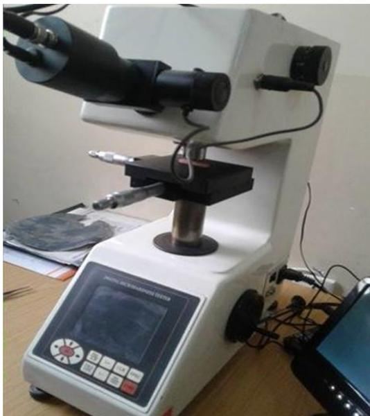
Fig. (4): Michrohardness test machine.
