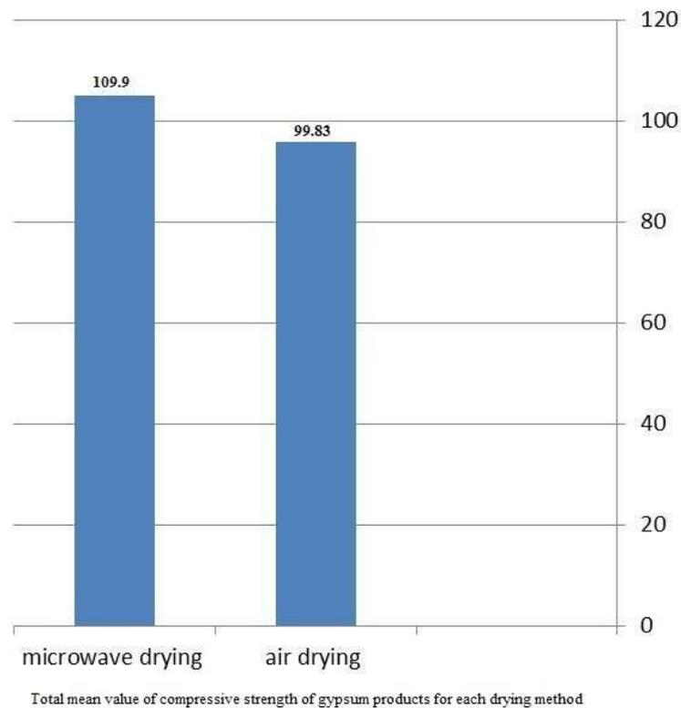
Total mean value of compressive strength of gypsum products for each drying method
