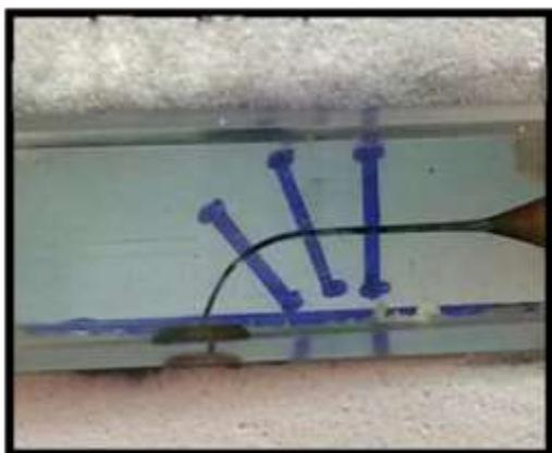
Fig. (1): Resin block in a Teflon holder.
