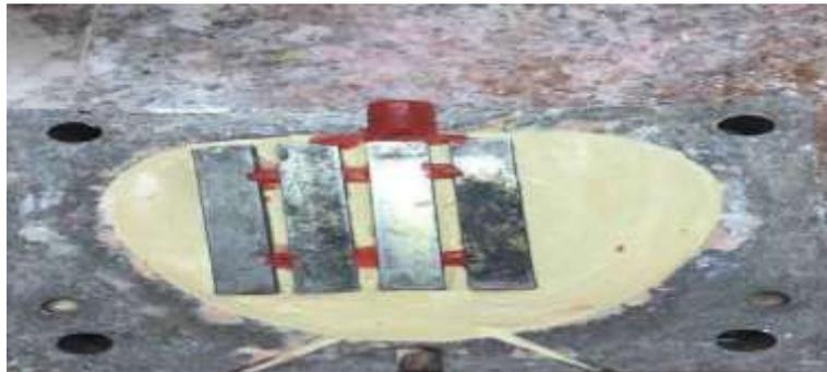
Fig. (1): wax sprues attached to metal patterns.
