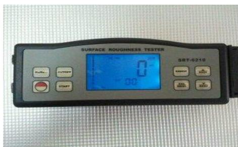
**Figure (5):** Surface roughness tester device
