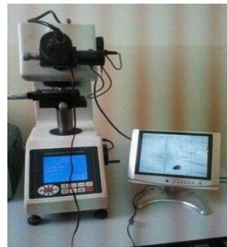
**Figure(6):**Digital micro hardness tester device
