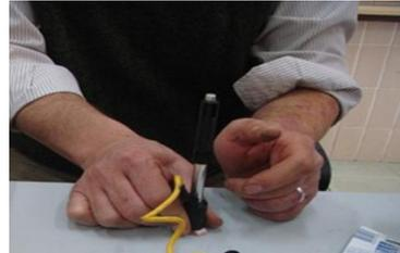
Fig. (4): Durometer hardness tester.
