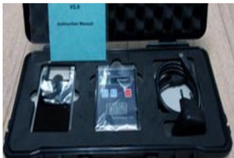
Fig. (5): The Profilometer device.
