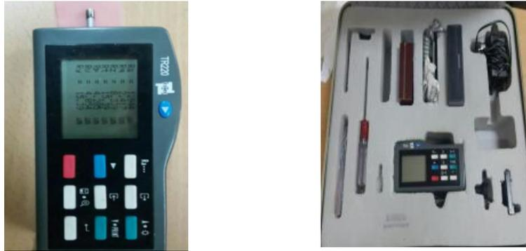
Fig.(4): roughness tester
