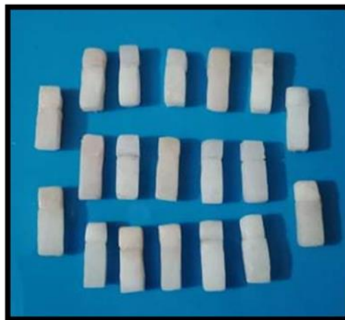
Fig. (4): Shear bond samples linked by using Glass ionomer cement.
