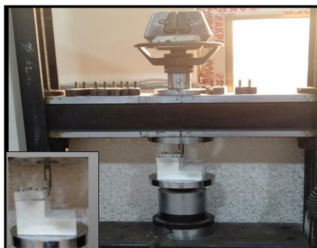
Fig. (5): Instron-1195 testing machine, the sample in holder and mounted in a universal testing machine.
