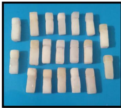
Fig. (3): Shear bond samples linked by using Breeze self -adhesive resin
