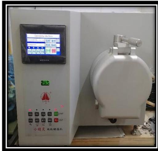
Fig. (3): casting machine for titanium alloy
