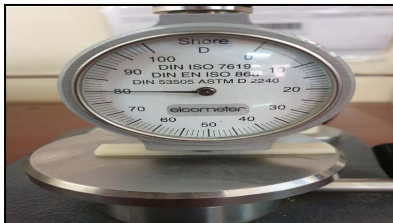
Fig. (5) hardness device (Shore-D)
