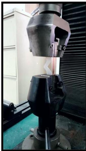
Fig. 2: Tear specimen mounted in the Universal testing machine.
