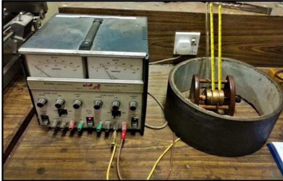
**Fig. (2): Thermal conductivity apparatus (Lee disc)**
