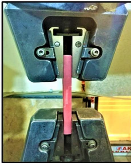
**Fig. (6): Instron testing machine during test the shear bond strength specimen**
